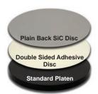
Double sided adhesive discs are adhered to a standard platen and used to secure plain back silicon carbide abrasive discs. Each provides 25-75 disc pulls, depending on grit size, cycle time and force.
