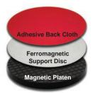
These reusable ferromagnetic stainless steel discs feature a nonslip backing and allow adhesive backed cloths/abrasive discs to be changed quickly and easily when using magnetic platens.
