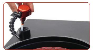
Retractable coolant nozzles allow quick and easy sample/bowl cleaning.
